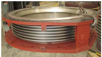
A 32" diameter hinged expansion joint with a C-276 van stone bellows
