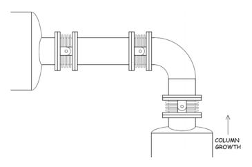
The pinned hinges allow rotation of the expansion joint while absorbing the pressure thrust - no main anchors are needed. Large piping and vessel thermal growth movements produced by FRP are easily accommodated by these rotation points.
